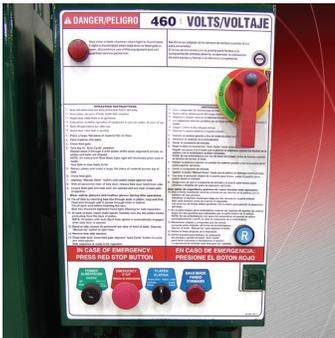
Standard controls: Key Lock On/Off Auto Cycle, Emergency Stop, and Platen Raise/Lower. Baler Ready light indicates the unit is operational. Shown with optional "Bale Made" light and electrical disconnect.
