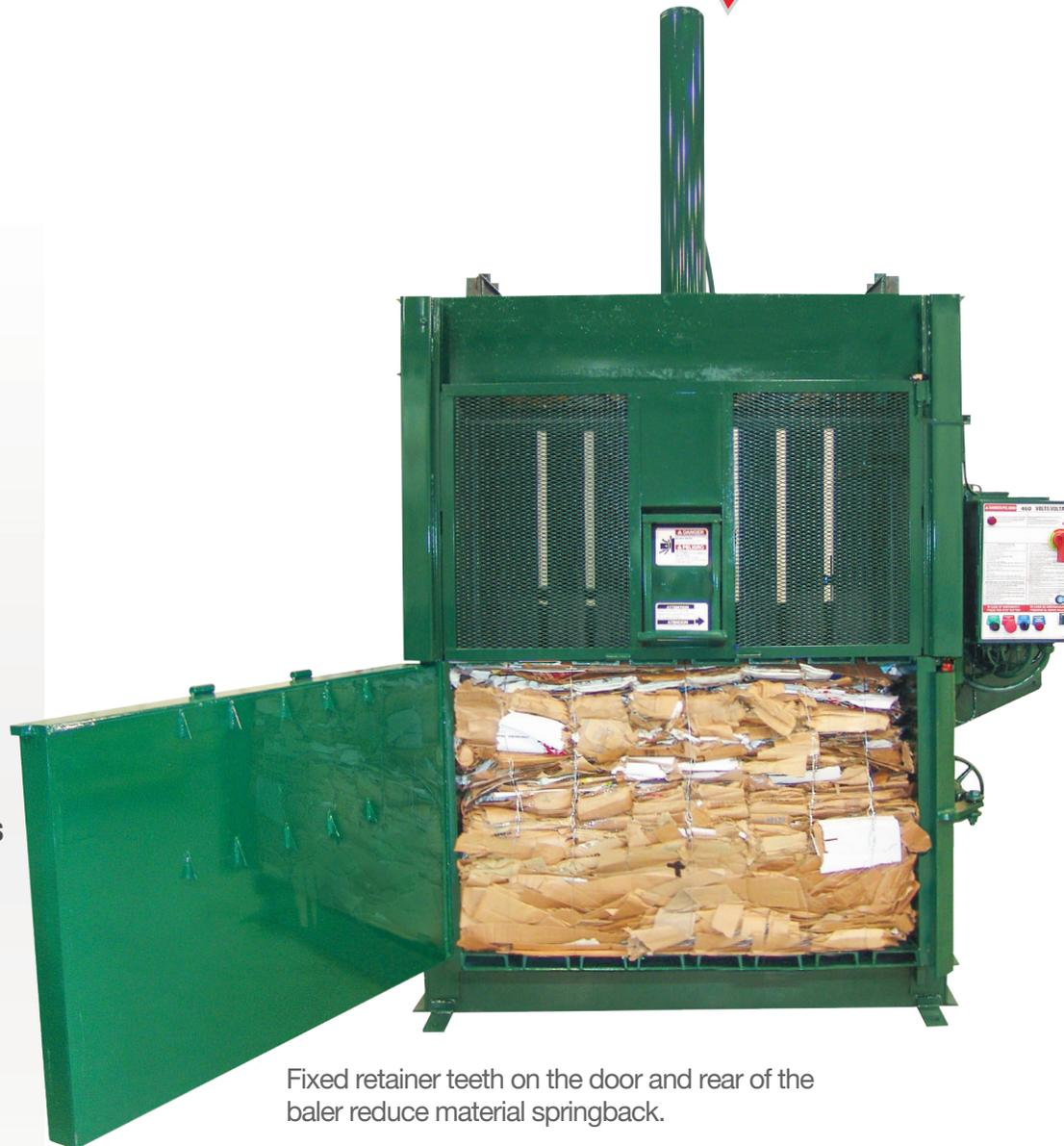
Fixed retainer teeth on the door and rear of the baler reduce material springback.
