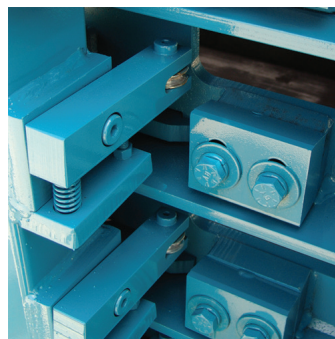
Spring-loaded retainer locks, adjustable wire positioners, and adjustable inserter needle positioners.
