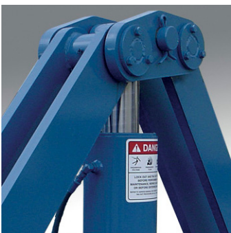
Single-cylinder bale tensioning system with linkage bars provides up to one million pounds of extrusion force.
