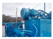
The advanced **Marathon** power pack is designed so that all of the valves are contained in a single manifold, which minimizes the number of hose connections and potential leak sources.
