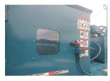
The chute feed hopper with inspection door and interlock switch will accommodate optional pneumatic, gravity, or conveyor feeding systems.
